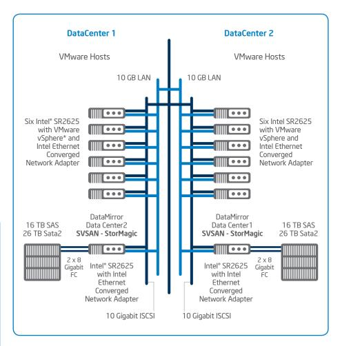
Systems SR2625, each with two six-core Intel Xeon processors 5600 series and 96 gigabytes (GB) of RAM. Servers are used for file, web, application, and database servers, supporting 48 applications and four databases in a VMware High Availability (HA) cluster. The environment is mirrored across the two data centers.
